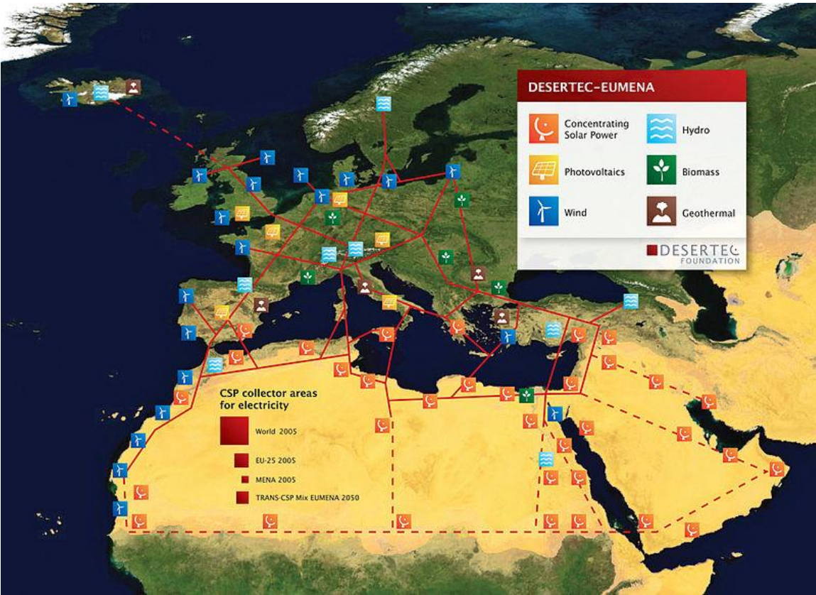
Figure 4. Hypothetical infrastructure of HVDC power supply in Europe, the Middle East and North Africa. Source: German Aerospace Center (DLR) Institute for Technical Thermodynamics (ITT)
